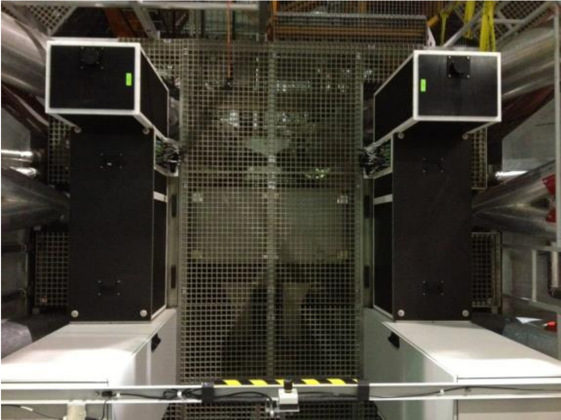
Large Binocular Telescope at Horizon - Preparing ARGOS S Laser Boxes for Alignment with Large Aspherical Lenses (LALs)
