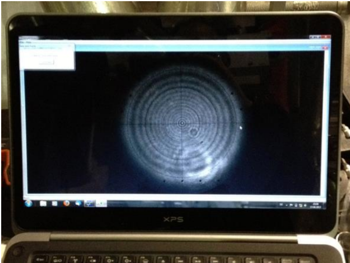
CCD Output Showing ARGOS Alignment Laser Properly Aligned With Respect To Large Aspherical Lens Target on SX Side of LBT
