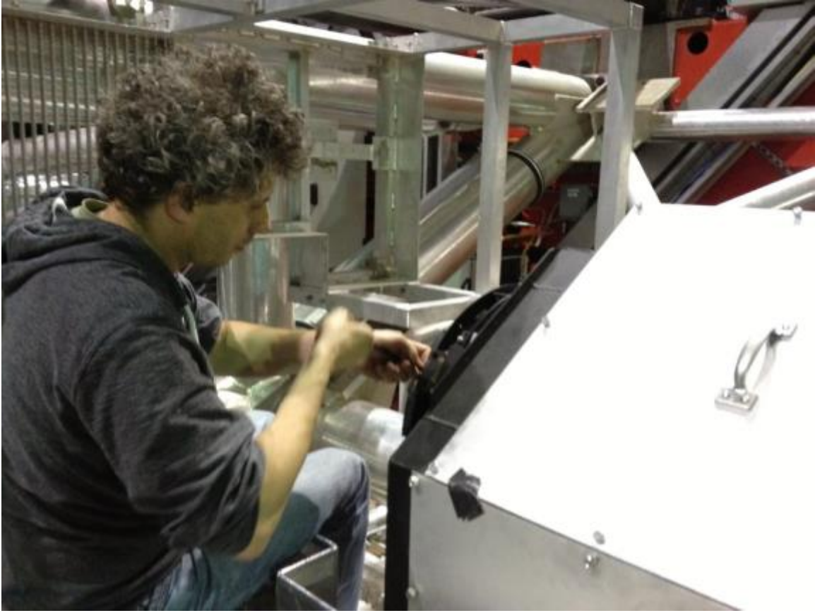
Tip-Tilt Alignment of Large Aspherical Lens on SX Side of LBT
