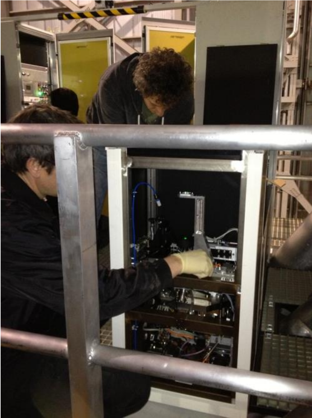
Verification of Internal Beamtrain Alignment Within DX Laser Box
